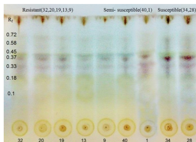
Figure 1. Profile of the band spots of purified saponins extracted from aerial parts of 9 alfalfa genotypes (mentioned in Table 1). Saponins were incubated with inactive enzymes during 12 h at room temperature.
